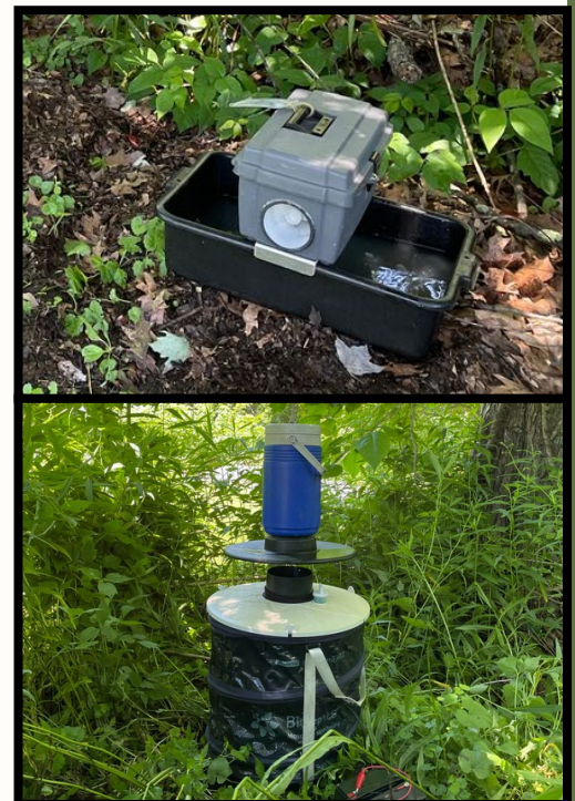
Figure 1. Two trap types that capture mosquitoes for surveillance and testing. Top: Gravid Bottom: BG Sentinel
